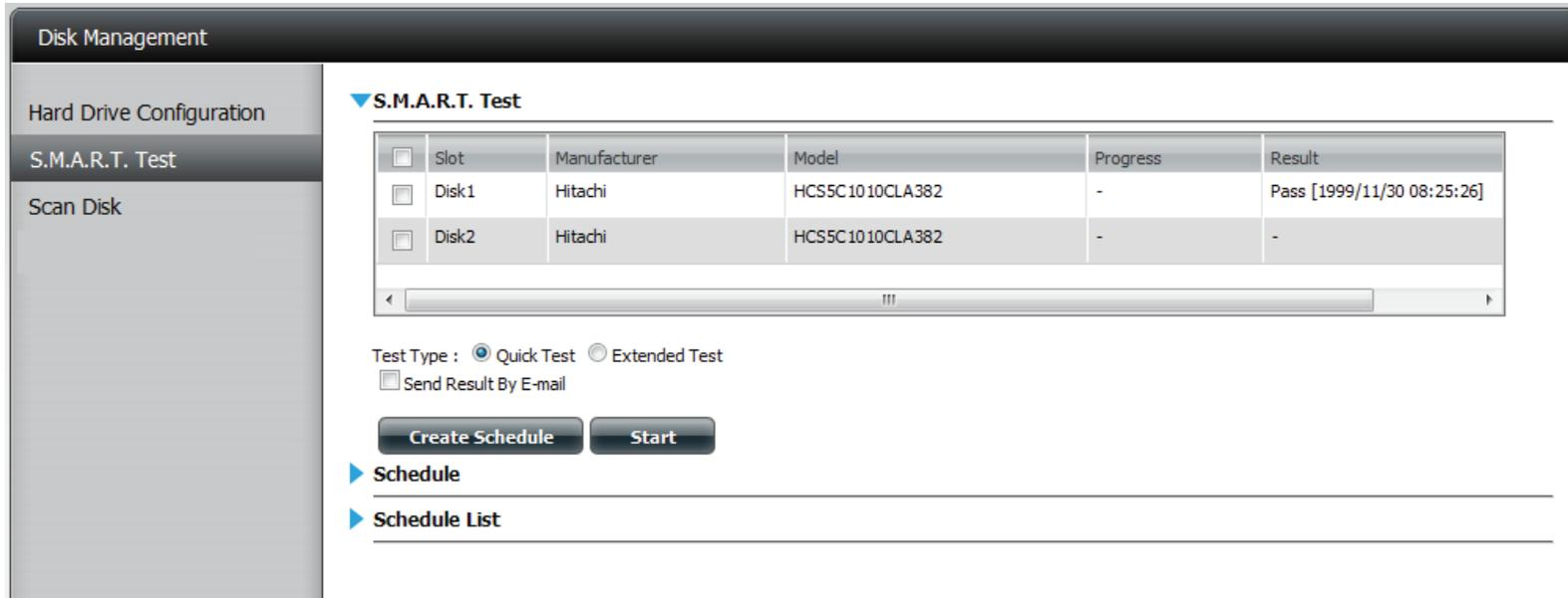
The screenshot displays the 'Disk Management' interface with the 'S.M.A.R.T. Test' section expanded. A table shows the test results for two disks. Below the table, there are options for 'Test Type' (Quick Test selected, Extended Test unselected) and 'Send Result By E-mail' (unselected). Two buttons, 'Create Schedule' and 'Start', are visible. Below these are expandable sections for 'Schedule' and 'Schedule List'.
